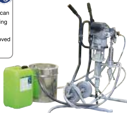
Hose system cleaning with PROLAQ Liquid
