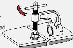
Use the rear slot on the Half Clamp to easily break off the coupon.
