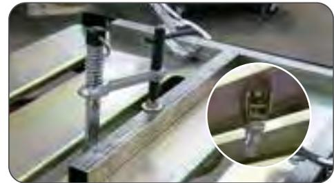
The MagSpring™ Clamps can be inserted into the 1.1" slots on the Nomad™ Tabletop for hold down clamping. Magnetic V-Pad jaw holds underneath the table to keep the clamp in the up-right, "ready to use" position.
