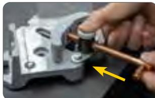
Press and hold the **Quick Acting Button** and the spindle assembly slides in and out for a super fast set-up!
