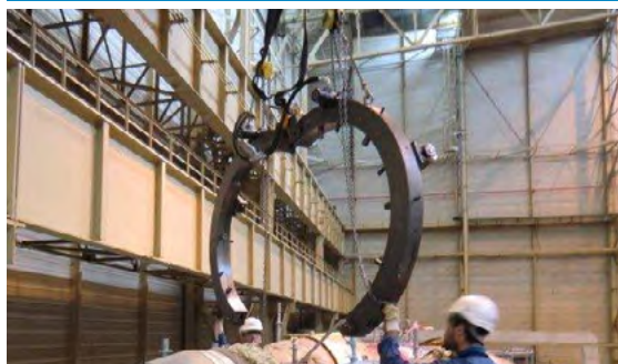
TT1400 Cutting and beveling machine with pneumatic drive
