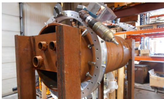
TT900 Cutting and beveling machine with pneumatic drive
