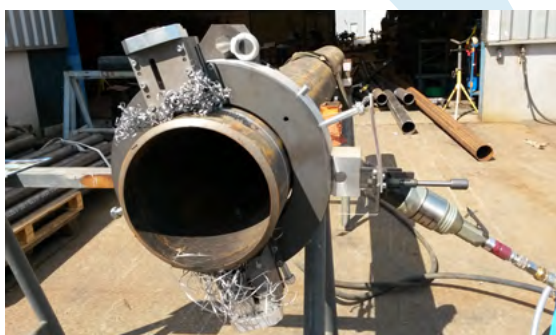
TT273 Cutting and beveling machine with pneumatic drive
