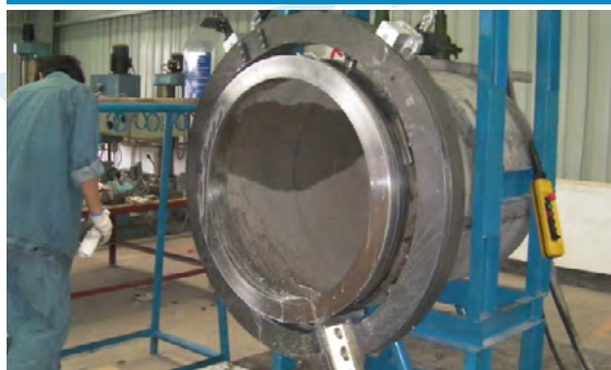
TT1016 Cutting and beveling machine with pneumatic drive
