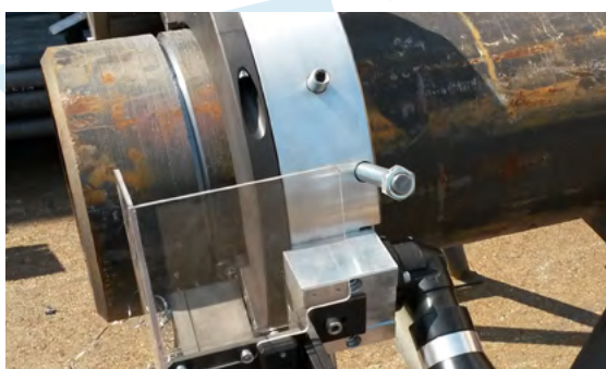
TT219 Cutting and beveling machine with pneumatic drive
