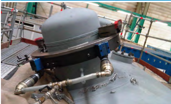
TT508 Cutting and beveling machine with pneumatic drive
